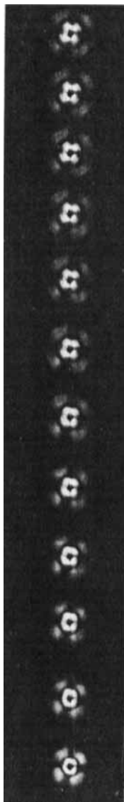
FIGURE 11 Observed optical pattern of dark ring in Case 1 of stage II. p = 5 cm Hg, \Delta t = 0.03 s.
